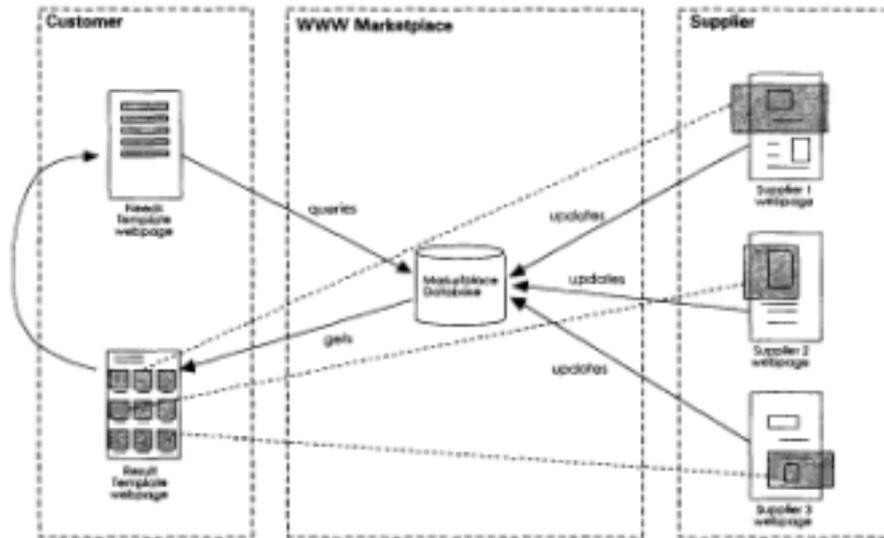
Figure 2. Architecture of the WWW electronic marketplace developed at the Harvard Design School. The efficiency of the marketplace design derives from the combination of optimized distribution of critical product/expertise data and the use of semi-formalized templates.
