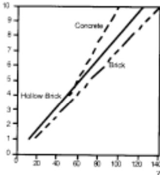
Figure 8. Relationship between the thermal resistance incremental factor (Z) and moisture content (uv).
