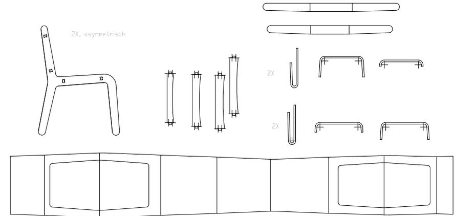
Fig. 24: cutting plan for the 1:1 model (p. 25), the plan is linked to the 3D model. if any measurements change in the 3D model, they are automatically changed on the plan !
