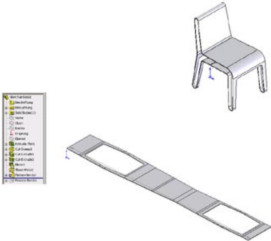
Fig. 23: folded and unfolded skin with the SW feature tree
