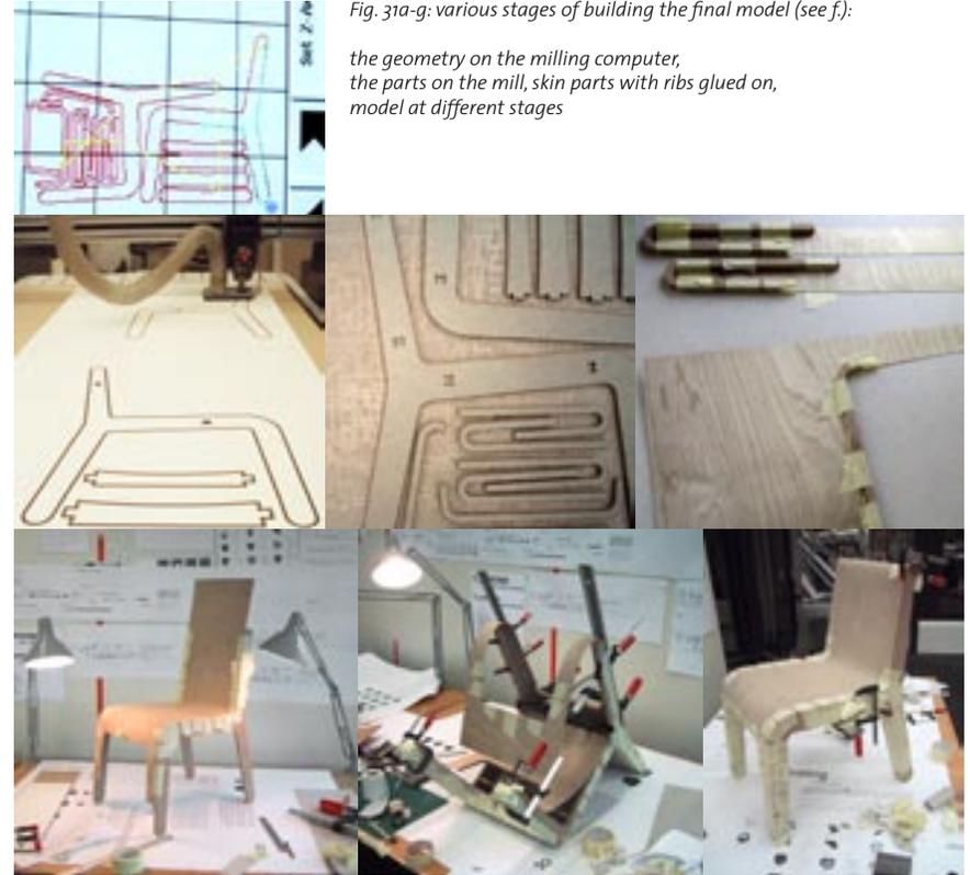
Fig. 31a-g: various stages of building the final model (see f):
