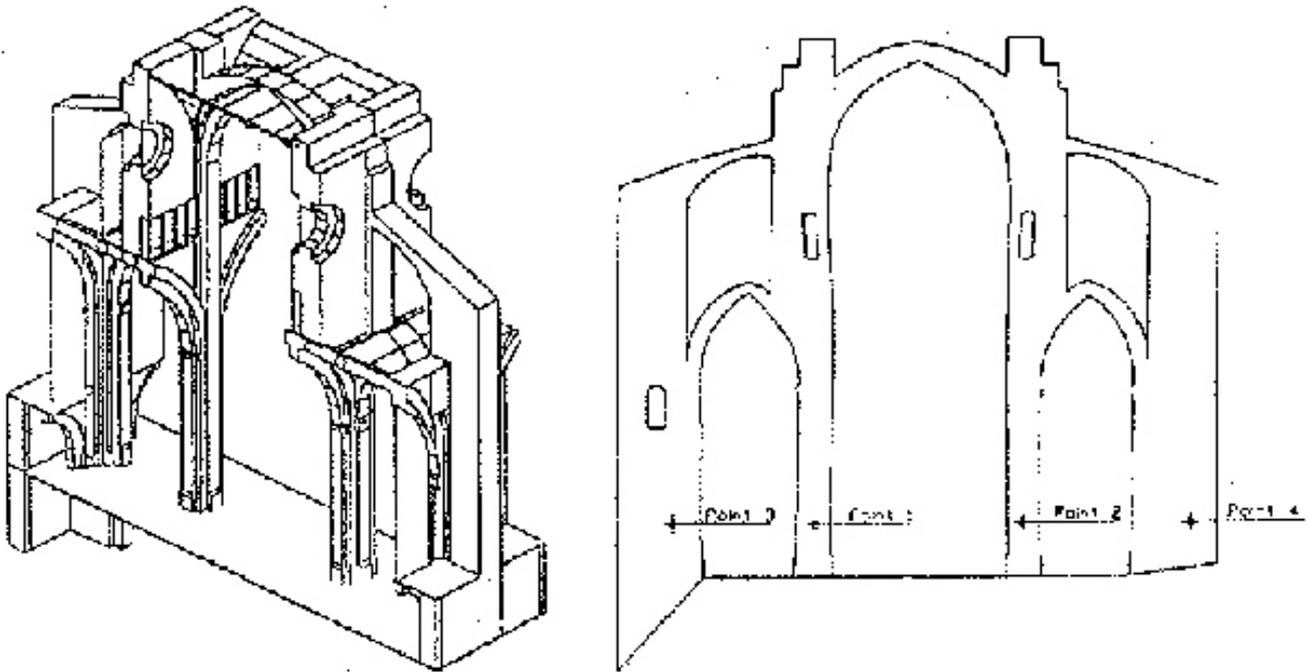
Fig. 5 - Measurement points using the "Hole Drilling" method.
