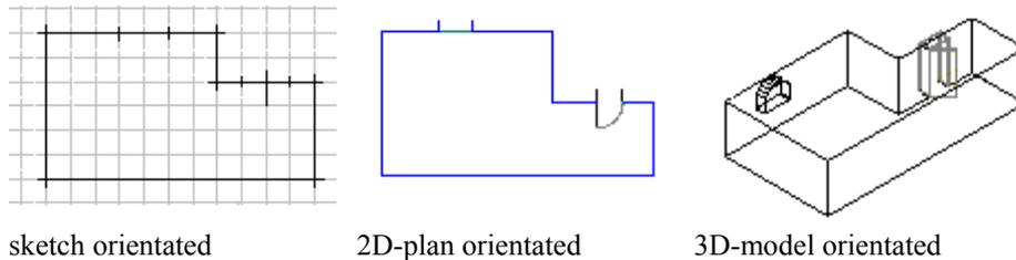
sketch orientated                      2D-plan orientated                      3D-model orientated
