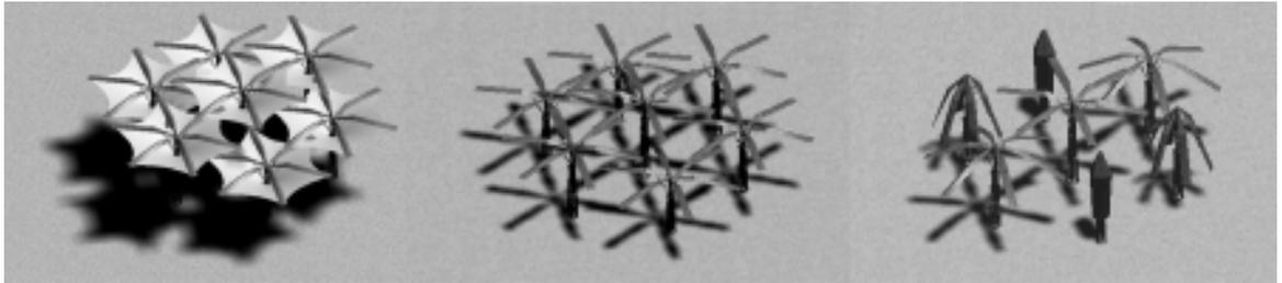
Figure 4. Multi-unit structure: Pattern of closing and opening umbrella units to avoid collision of parts.
