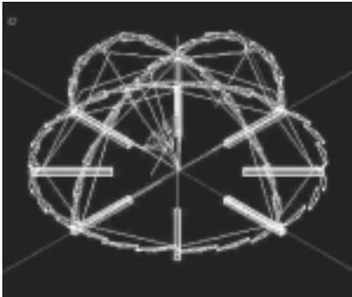
Figure 2. Spherical scissor structure (C. Hoberman design).
