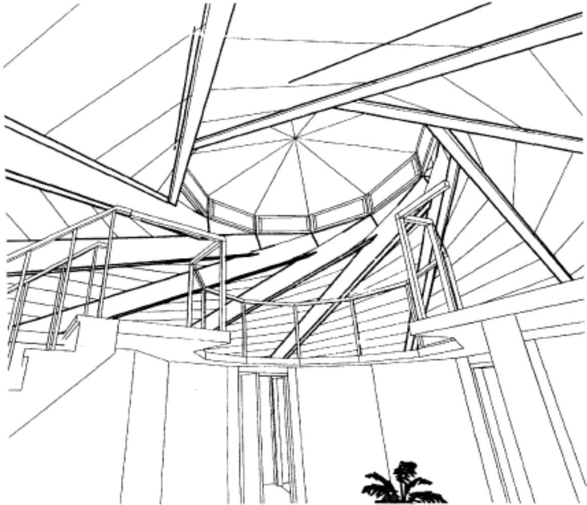
Figure 4. Interior view of Reciprocal Frame roof for a house
