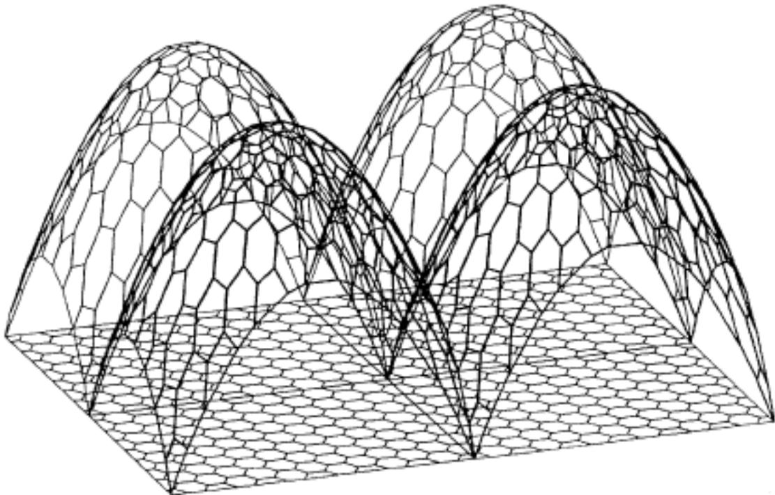
Figure 7. Example of the "clean" connection line between faceted paraboloids with a regular hexagonal pattern on the horizontal projection plane.
