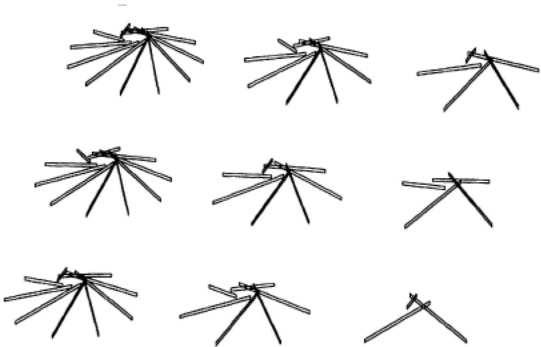
Figure 2. Examples of computer generated Reciprocal Frame configurations
