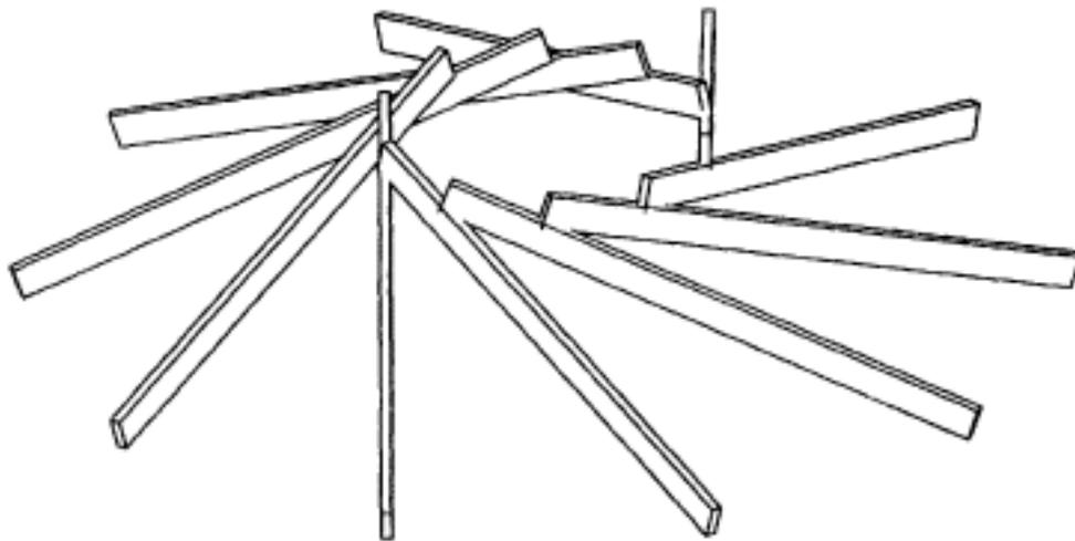
Figure 1. A typical Reciprocal Frame 3-dimensional beam grillage.
