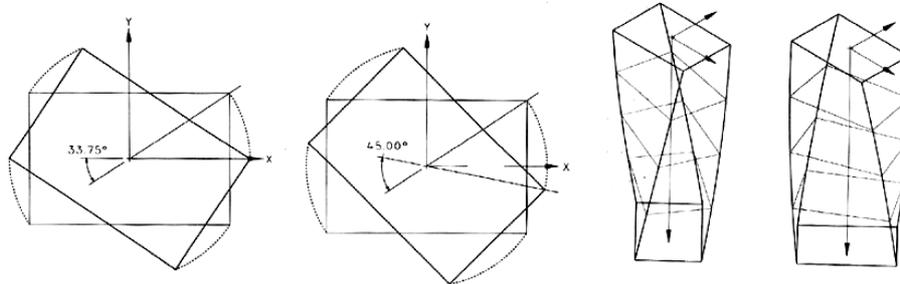
Figure 1: 'rectangular' column-modelling technique: Counter-rotation of two rectangles with a translation along the z-axis
