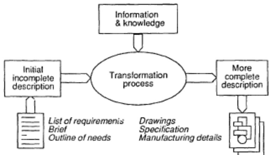
Figure 1. Designing viewed as a process of transformation where an incomplete description of an artefact is progressively changed to a complete one by the use of knowledge and information.
