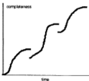
Figure 3. Plotting the progress of a design overtime results in a graph with discontinuities arising where new ideas supplant old and temporarily set back developments.
