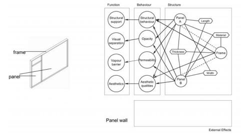
Figure 1. A panel wall and its corresponding FBS representation
