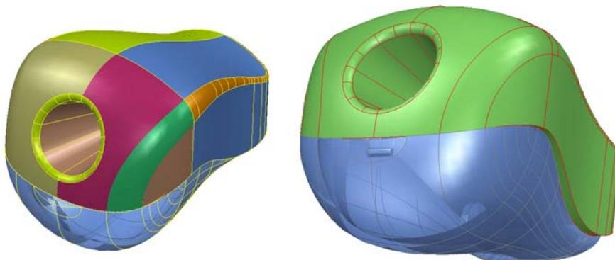
Figure 2. Drawings of the linked surfaces of a pencil sharpener.
