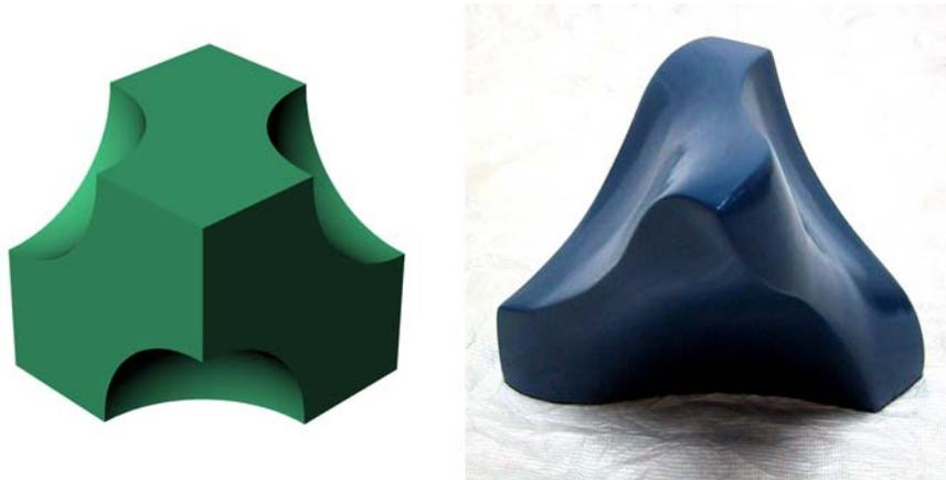
Figure 6. Student's design starting from the subtraction of four spheres from a cube. Selective fillets break the original symmetry and link some adjacent faces. Even though continuity is increased some edges are maintained that emphasizes the tension between smoothness and discontinuity.
