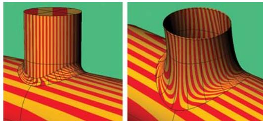
Figure 4. Continuity G1 in fillet surfaces and G2 in blend surfaces.
