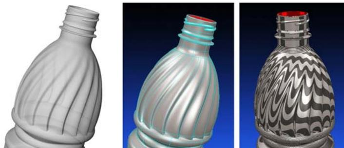
Figure 10. Perceptual discontinuities in a geometrically continuous bottle, as can be seen by the zebra analysis. Continuity of G2.
