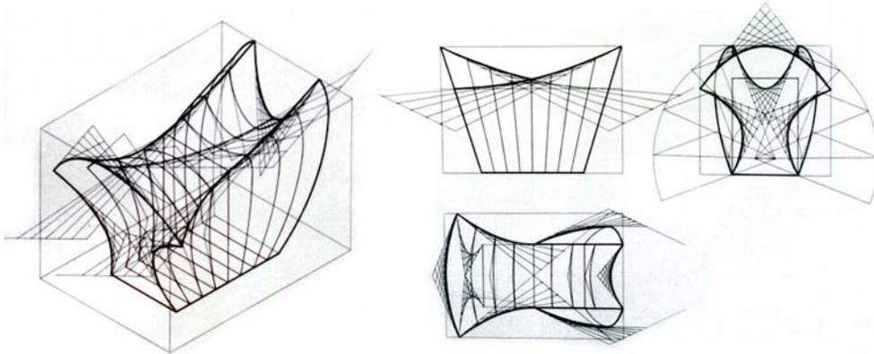
Figure 1. Surface that goes through a continuous transformation from convex to concave zones. Created by a student, Cardozo.
