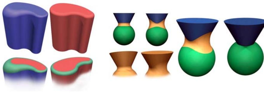
Figure 5. Fillets between a cylindric surface and its cap and between a cone and a sphere. The union is smoothed if the symmetry of both shapes is diminished by the linking surface.
