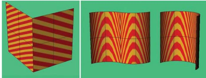
Figure 3. Zebra analysis of two planes in contact (G0), of two quarters of a cylindrical surface joined with an inflection line (G1. They share the tangent plane but curvature turns from negative to positive) and of two quarters of cylindrical surface joined with tangent and curvature continuity (G2).
