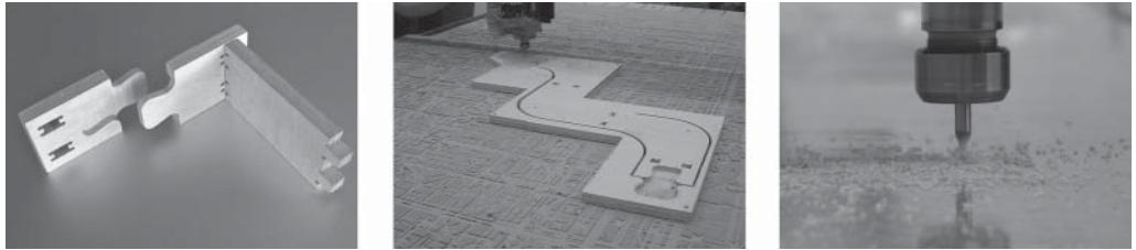
The structural data was concurrently imported into the software Maya, where it was pre-processed for fabrication by a MEL script program, and then exported for G-code processing.
