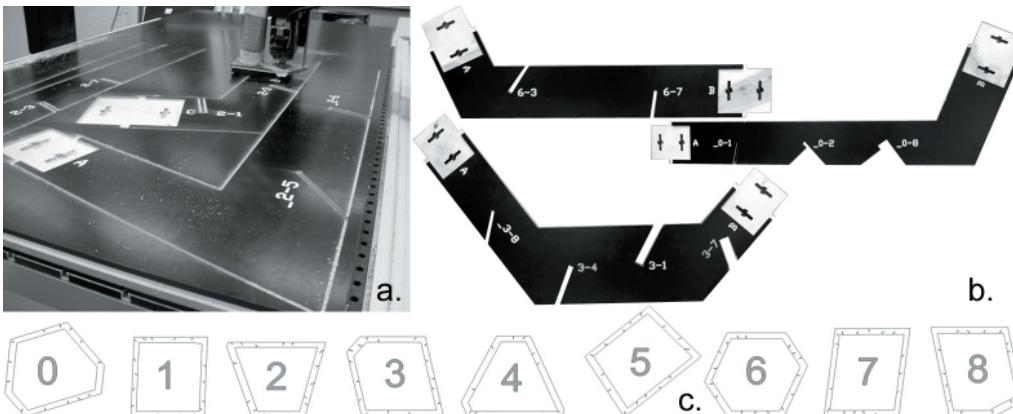
Figure 4. Production process. (4a) elements were cut by 3-axis milling machine; (4b) elements of the frame with engraved descriptions; (4c) set of frames for the prototype;
