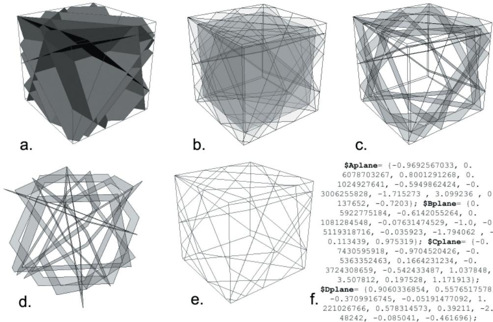
Figure 1. General idea of the structure. (1a) freely rotated planes inside a cube; (1b) subtraction of an inside form; (1c) frame structure with wireframe visible; (1d) frame structure; (1e) linear representation for calculation purposes; (1f) mathematical description of a frame set (four coefficients for every frame).
