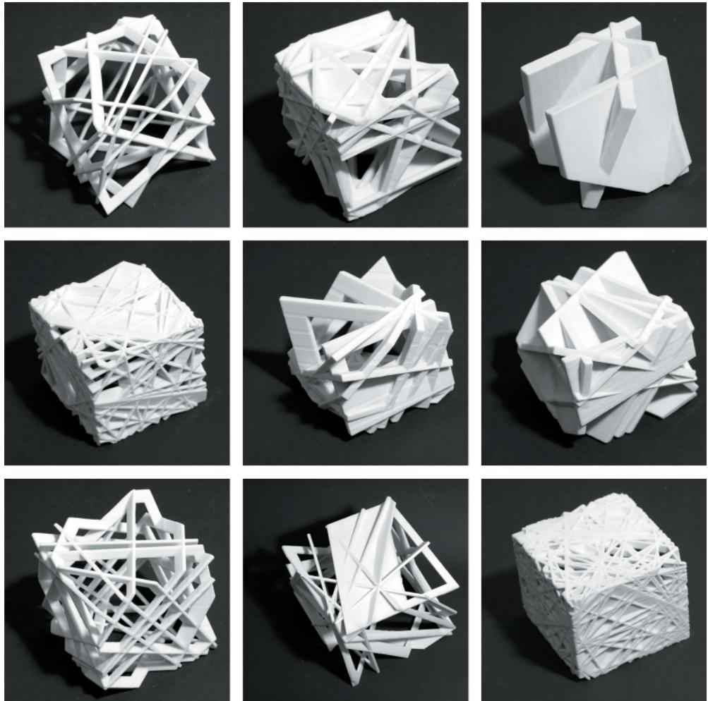
*Figure 2. Examples of different cubes produced by a plaster 3D printer – showing different densities of the grid as well as a variety of possibilities offered by changing the frame thickness and proportions between the outside and inside cube.*
