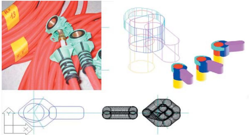
Figure 2. CAD-Chain: 3D-modell and CNC-milling-paths and steps for the tubes
