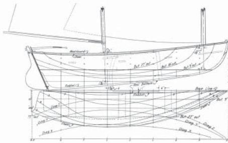
Figure 3. Lines of 17-Foot Hampton Boat from Chapelle, H.I., *Boatbuilding Boatbuilding*.1941
