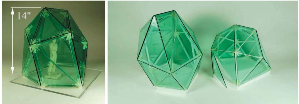
Figure 8 Final models assembled of laser cut acrylic sheets, laser cut members, FDM finger joints and glass clips printed of abs plastic.
