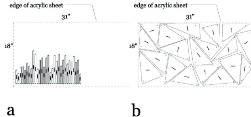
Figure 7 (a) file for laser cutting member (b) file for laser cutting glass panels
