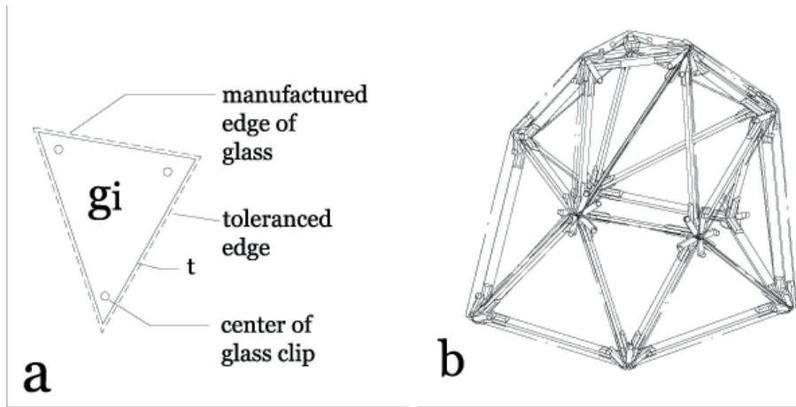
Figure 5 Parameters for glass panel (a) and a fully installed model of assemblies, structural members and glass components (b)
