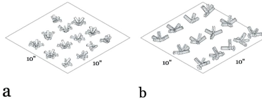
Figure 6 (a) finger joints on print bed, (b) FDM printed finger joints with no support material above the printed joint, parts are positioned flat to the print bed
