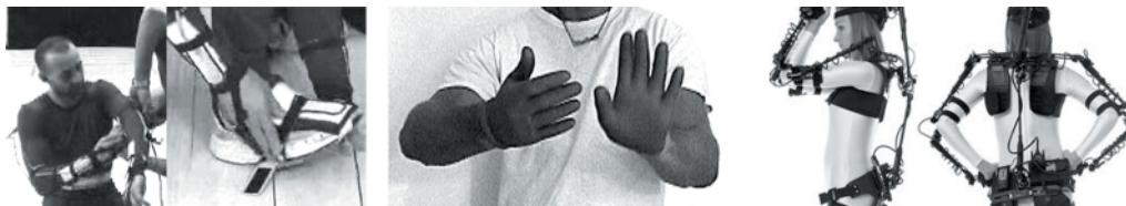
Figure 3. La Kitchen's 'Kroonde' wireless 16-sensor motion capture system (left) ([www.cycling.com/products/kroonde.html](http://www.cycling.com/products/kroonde.html)), color tracking of hand motion using Internet video camera (middle), and Animazoo's 'Gypsy Torso' motion capture suit (right) ([www.animazoo.com](http://www.animazoo.com)).
