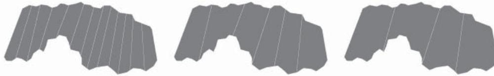
Figure 2. The land-parceling tool: different subdivisions of an area into equal size parts.
