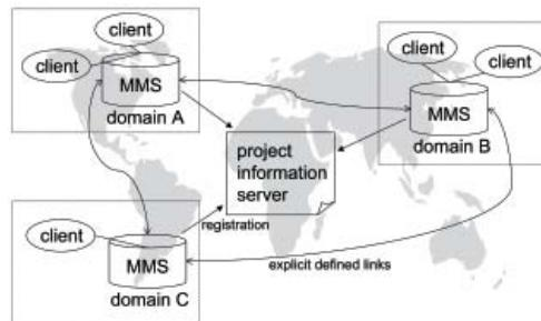
Figure 1. System architecture realized for the platform.
