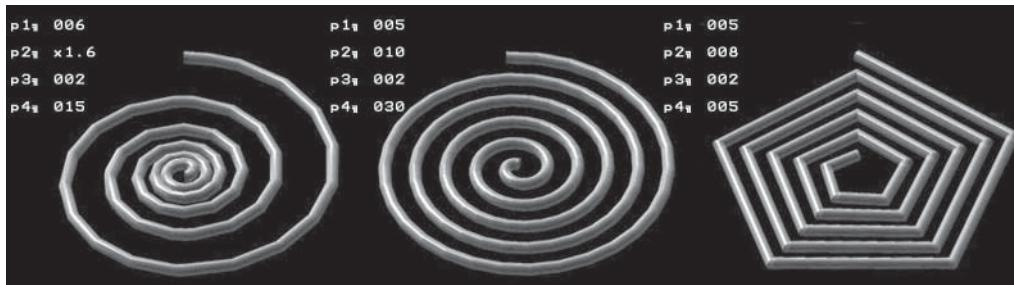
Figure 3. Render of spirals made with the program - a logarithmic spiral, an arithmetic spiral and a spiral made with a low quantity of segments. The number (1) corresponds to the number of turns; (2) distance between turns; (3) Extrusion ray; (4) Number of segments per turn - geometric resolution.
