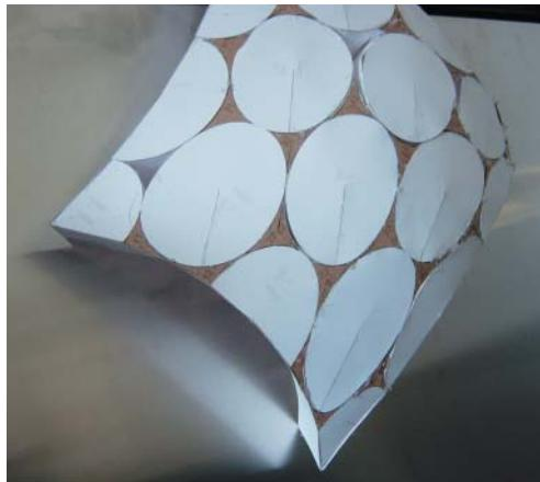
*Figure 4. Cone based approximation of a double curved surface using only developable surfaces*
