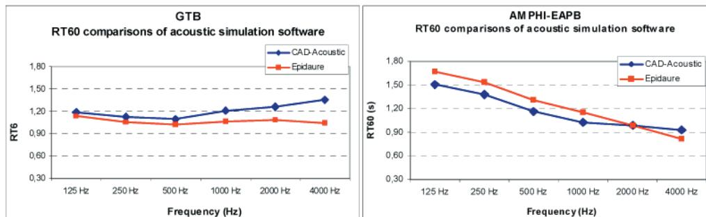
Fig. 11. Reverberation Time (RT60) comparisons of the Amphi (left) and the GTB (right) by using different acoustic software
