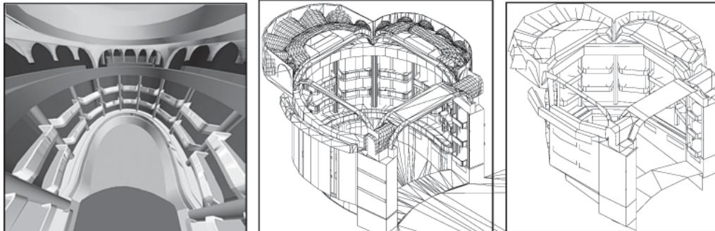
Fig. 5 – The initial model of the GTB (left) and the simplification from the most complex model n° 1 (middle) to the most simple one n° 4 (right)
