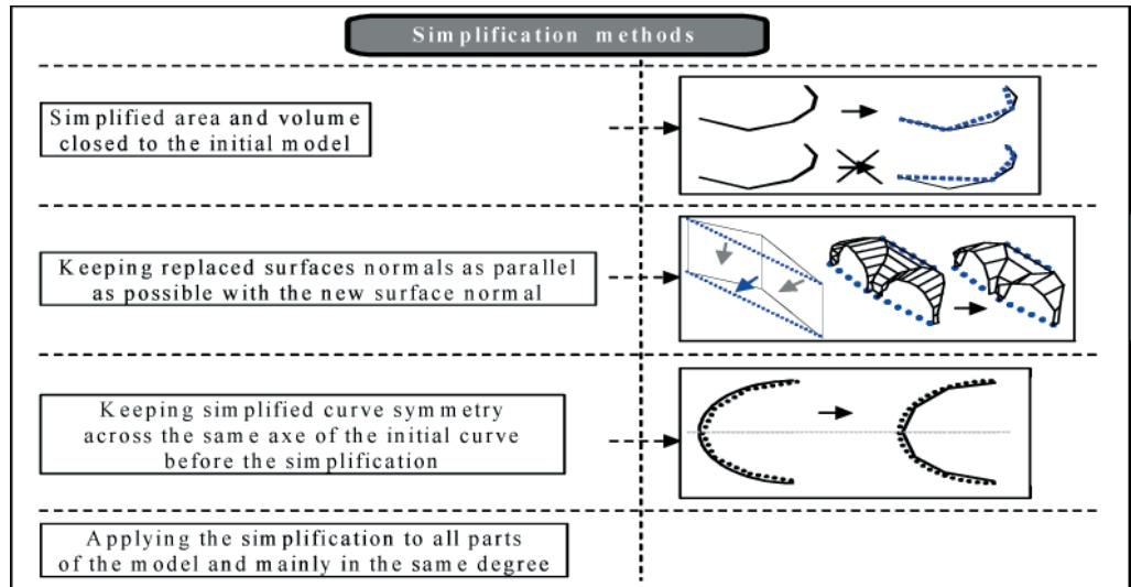
Figure 2. Simplification methods of models
