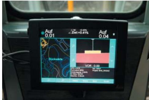
*In the driver's cab one can see the terrain model on the machine operator's display unit. The planning data is combined with the clear guidance data from real-time GPS positioning providing the machine operator with all the necessary details for the excavation, graphically and digitally, accurate to within a centimeter – more quickly, more comprehensively and more precisely than marker poles*
