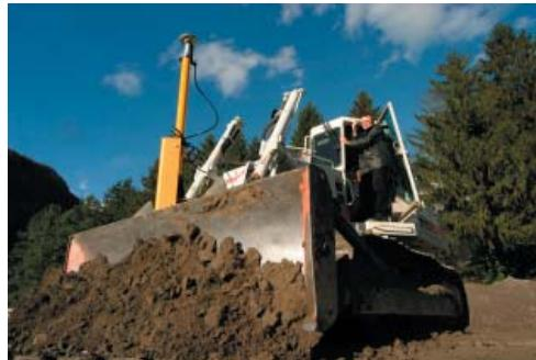
*The construction machine is equipped with a Leica Dozer system, which determines the 3D position of the blade in real time to the nearest centimeter. The driver of the machine receives all guidance details directly from the system.*
