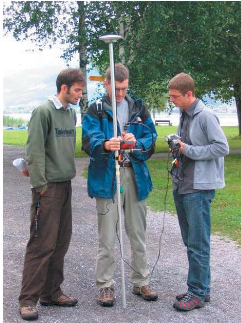
*Ergonomic test of Leica GPS-20*
