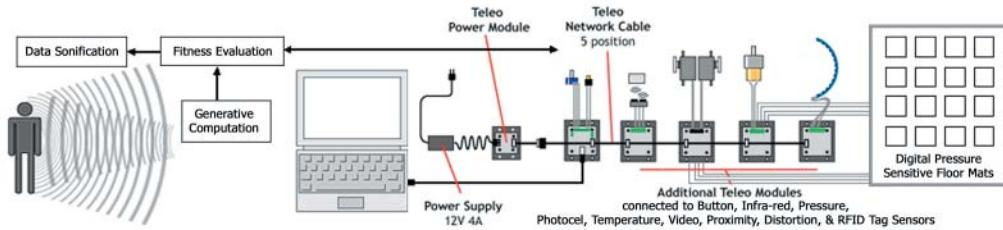
Figure 5. Sensate system: input from digital pressure sensor mats, infra-red, piezo pressure detection, temperature, light-sensitive photocells, proximity, RFID tags.
