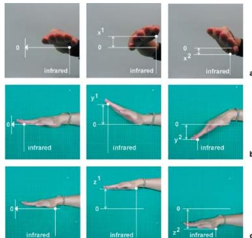
Figure 4. a. Use of arm rotation and palm movement to obtain X axis; b. Use of wrist rotation and palm movement to obtain Y axis; c. Use of palm elevation to obtain Z axis
