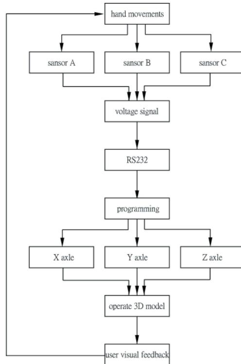
Figure 6. The HMS operating sequence
