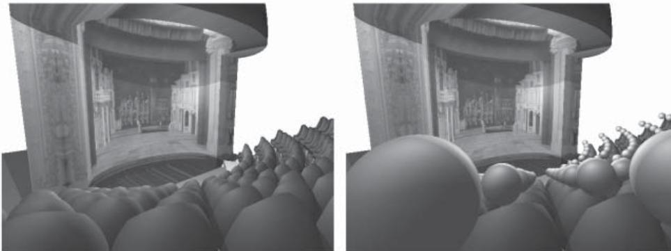
Figure 7. View of a scene and seats in the model experiment and simulating the spectators.
