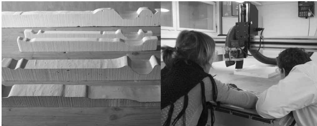
Figure 4 Plaster sections (left) & Pre- cix™ 3-axis CNC mill (right)
