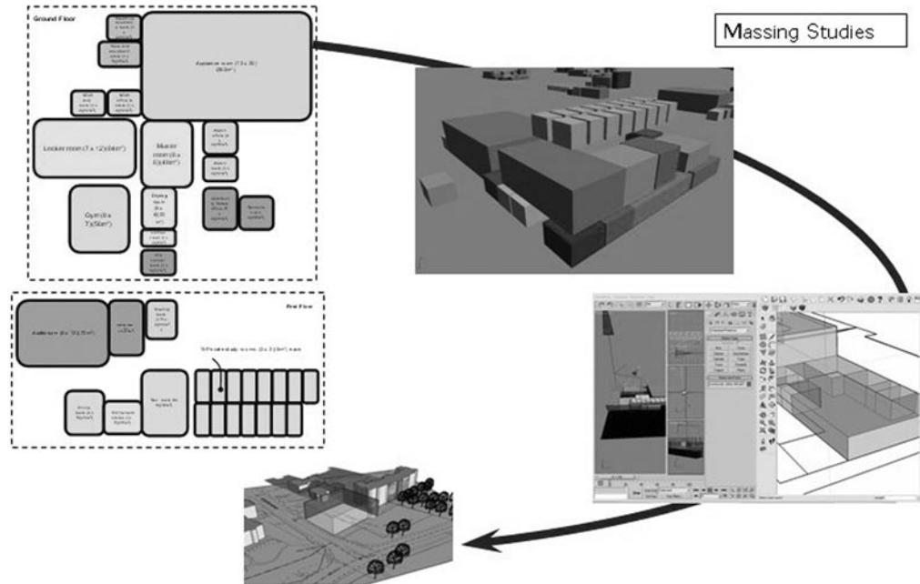
tion were imported from DigiMap so that the various buildings and rooms making up the fire station could be realistically positioned on site. A simple day lighting design was carried out in SketchUp to refine the room layouts for maximum functional and thermal efficiencies.
