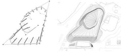
planar basis. The cones are implicitly derived by the edges of the planar faces and the constraint of tangency (Figure 4).
