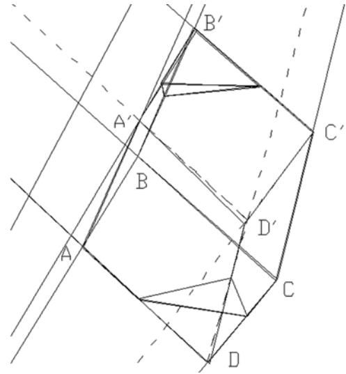
this hypothesis. A proposal of a parallelepiped close to the polyhedron of the engraving is given. In figure 4 (left), the positions of the vanishing points of the directions of edges (pf1, pf2 and pf3) are given. The orthocenter h of the vanishing points is outside of the triangle (pf1, pf2, pf3). That means that the three directions are not orthogonal. A comparison with
