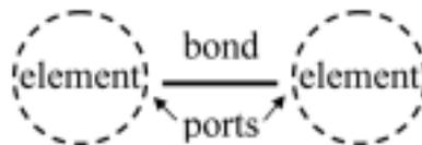
Figure 2. Bond and ports of bond graph.
