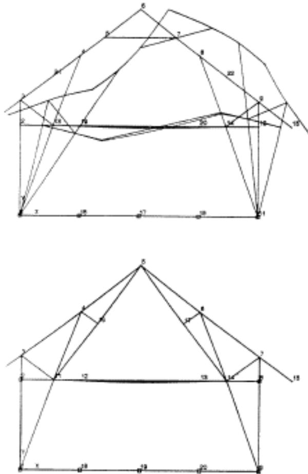
Fig.4 Deformed shape of timber-framed house under lateral wind loading (a) original design (b) proposed solution
