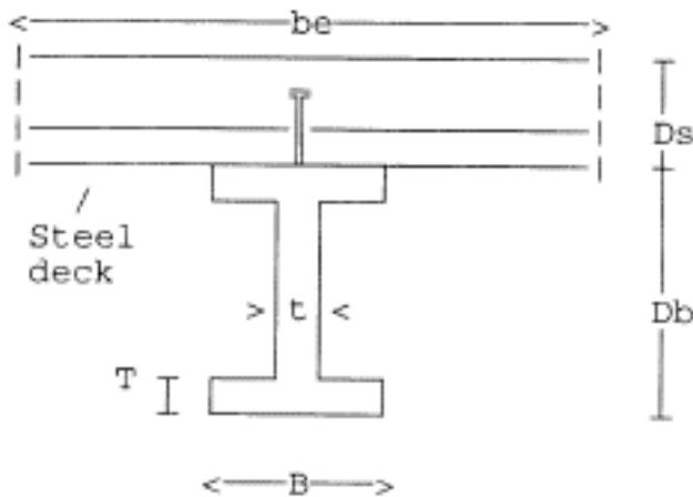
Composite steel deck floor - Internal beam U.D.Loading
