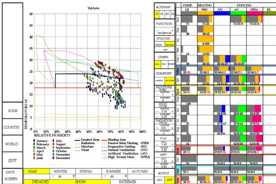
Figure 8. The bio-climatic chart for residential buildings and the space of simple solutions for the thermal comfort design strategies.
