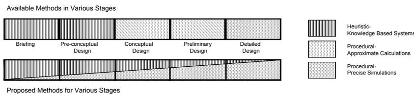
Figure 1: Schematic comparison of available vs. proposed energy evaluation tools in different design stages (from Shaviv and Kalay, 1980).
