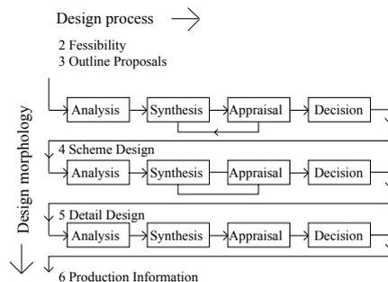
Figure 3: Basic scheme of a design process and its main activities (from Maver, 1971)
