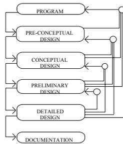
Figure 2: The Iterative Design Process
