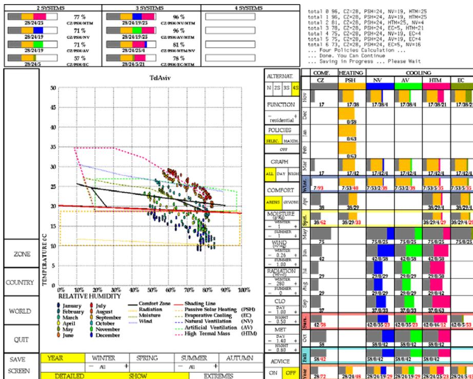
Figure 9. The bio-climatic chart for an office building and the space of simple and complex solutions for the thermal comfort design strategies.
