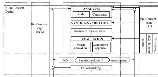
Figure 6: Basic scheme of the main activities in the pre-conceptual design stage
