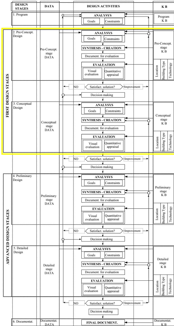
Figure 4: Basic scheme of a design process, main activities, knowledge bases and data
