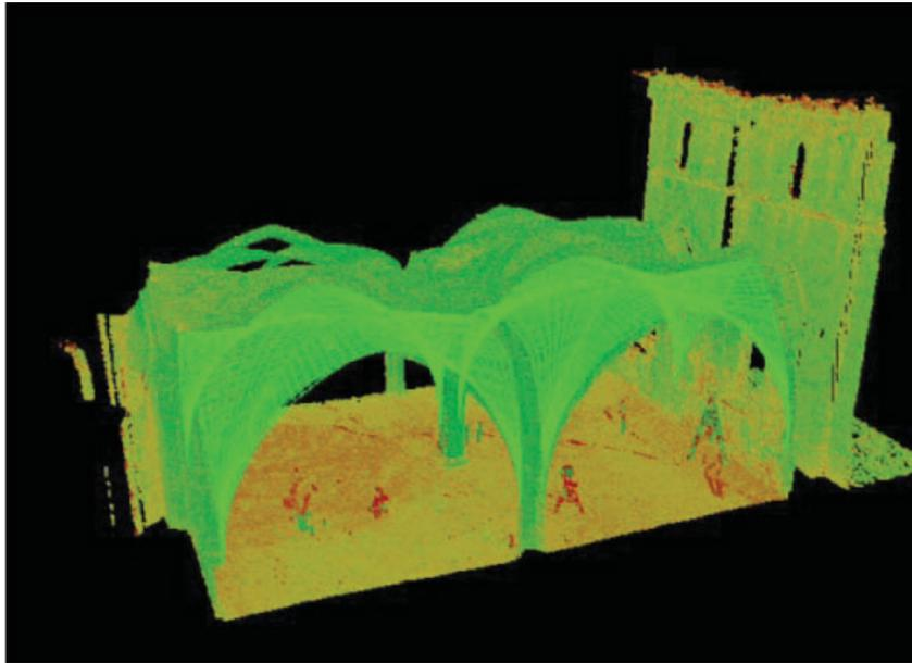
Figure 10. Refitting canonical geometry to the point cloud
