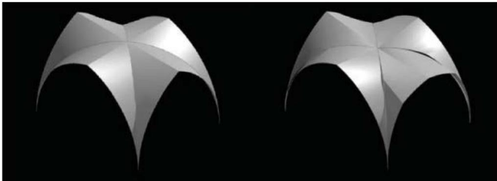
*Figure 9a and 9b. Canonical geometry in fully erect and hinged form.*
