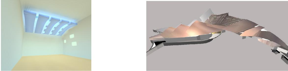
**Figure 4.** Art Museum Extension design by Kevin Stitak, Spring 2001. Radiosity software was used to test the regulation of daylight in a generic gallery space by ceiling mounted mechanical louvers (left). Decisions were made about the spacing, the materials and the size of the louvers, and the proportion and orientation of the openings. This was simply plugged onto the designed building without retesting the final designed space for daylighting (right).
