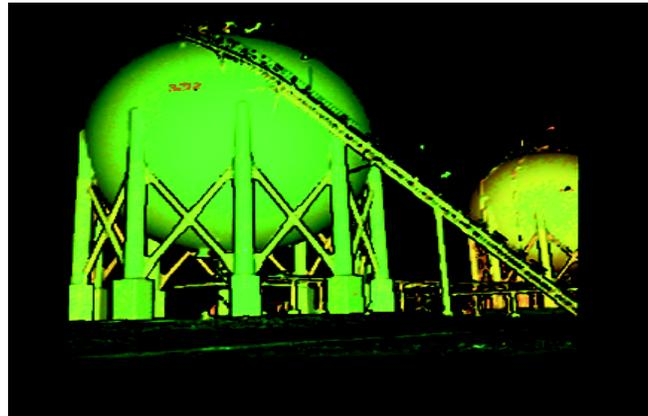
Figure 7. Cyra Technologies example laser scan of a full size refining facility.
