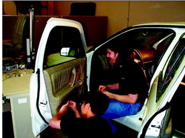
Figure 1. Taping datum lines on a car. Photo Courtesy of 3Name3D.
