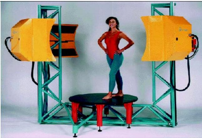
Figure 4. A Cyberware laser scanner.
