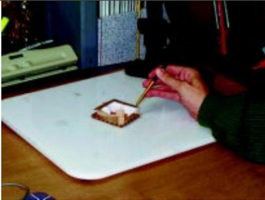
Figure 9. Digitizing the physical model with the stylus.
