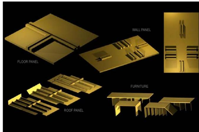
*Figure 1. CAD 3D model of shelter components (Koh, Leng & Teo).*
