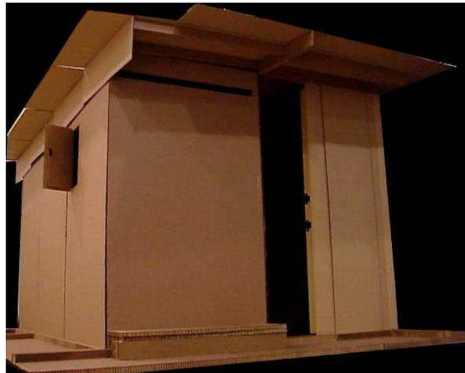
*Figure 5. Assembled full-scale shelter made of paper honeycomb board and corrugated cardboard (Koh, Leng & Teo).*
