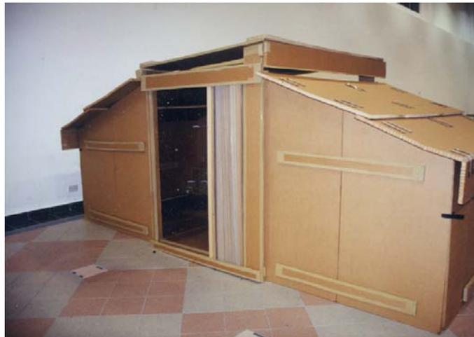
*Figure 7. Full-scale shelter made from corrugated cardboard and paper honeycomb board (Tan, Choy, Lim).*
