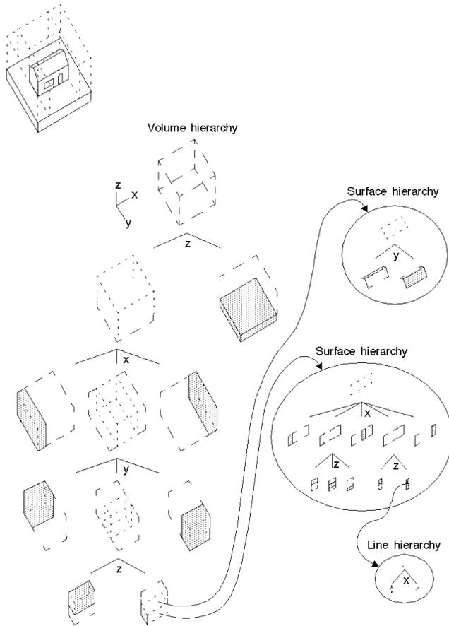
Figure 8. Example for hierarchical decomposition of a house
