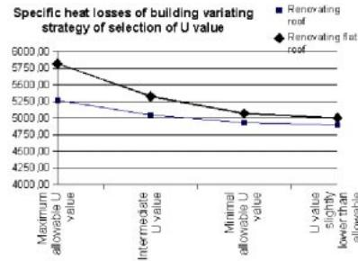
The values of specific heat losses for the first and second solutions are not very distinctive because of the relatively small difference between roof envelope areas. The third solution could be a rational proposal for the client to invest by purchasing the windows with better U-value.
