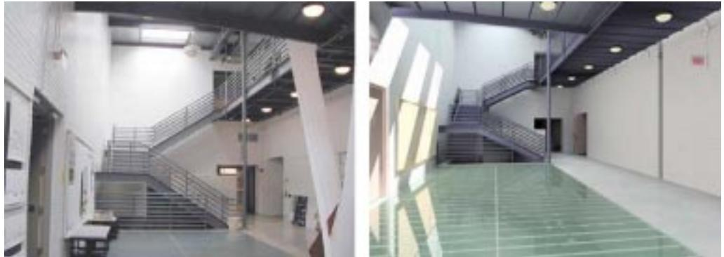
Digital cameras with wide-angle lens are then used to photograph the interiors of cardboard models under simulated daylighting conditions. Images of the interior spaces are available almost instantaneously for the designer to contemplate and adjust (e.g. widening an opening, or changing the curvature of a light scoop etc.).
