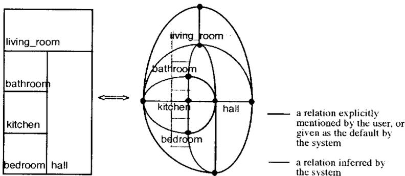
Figure 7 Graph Representation of a Planning Layout
