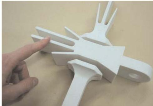
Figure 6. 3D printed house (scale 1:100) from plaster based powder.
