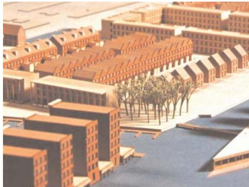
Figure 3 and 4. Laser cut facades (scale 1:1000) in 0.5 mm wood veneer.
