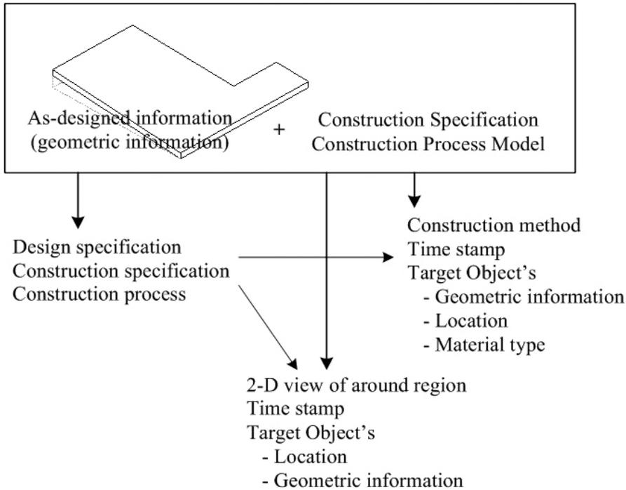
Figure 2. Different representational needs on a slab
