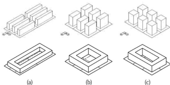
Figure 3. Layouts with 6 equal sized plots, nuclear and perimetral typologies
