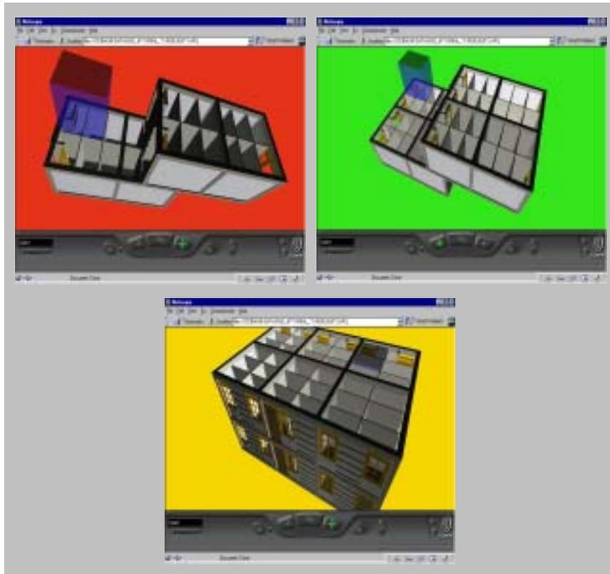
*Figure 5. VRML models as based for configuring housing unit, each is module with maximum area  $36\text{ m}^2$  (top left),  $72\text{ m}^2$  (top right) and  $108\text{ m}^2$  (bottom)*
