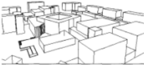
Figure 9 Perspective made in order to study the relationship with the surroundings of the designed mass (at the centre of the image). The impossibility of highlighting the mass, together with the lack of precision of the algorithm for the removal of the hidden lines, make this image of little use.
