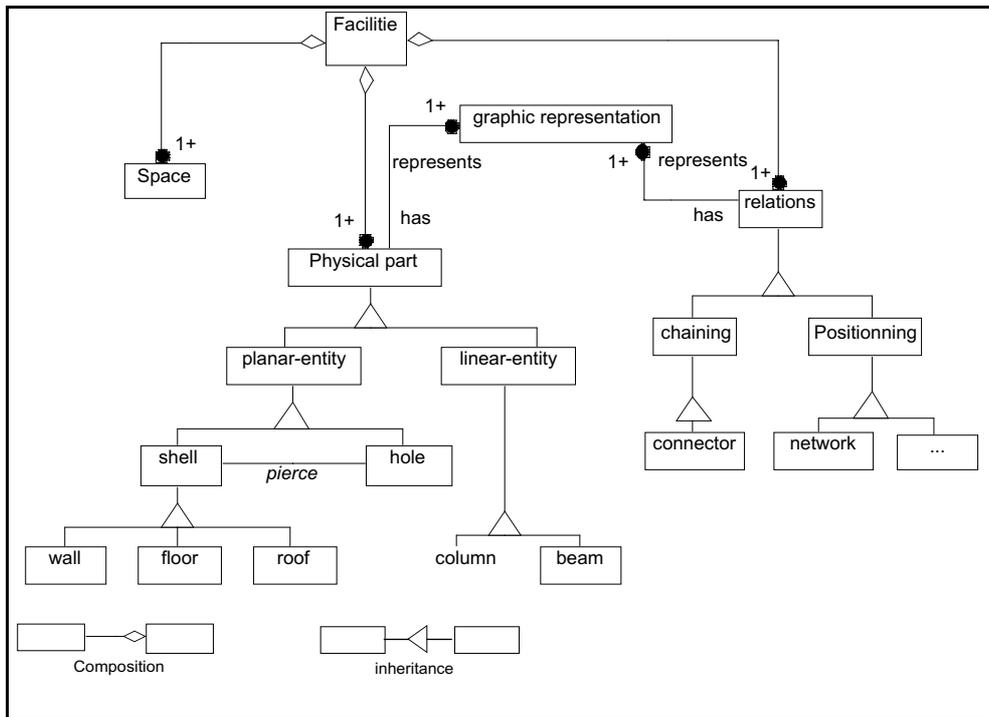
Figure 1: arTec model : design objects and relations.<sup>7</sup>
