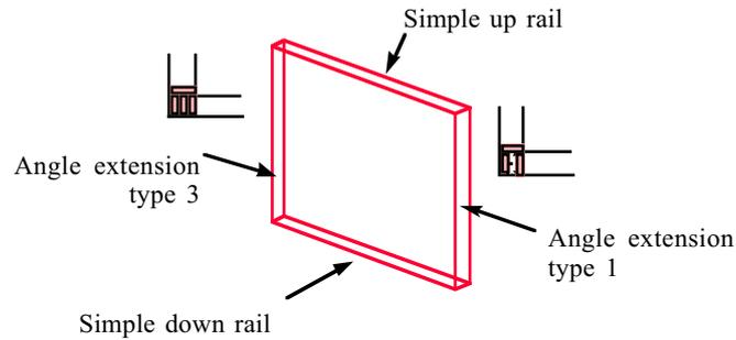
Figure 7: wall boundary characterization operation.
