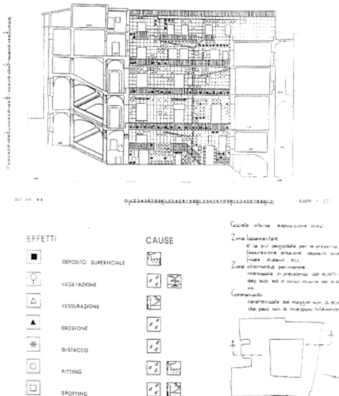
**FIG. 5** Localisation of the phenomena is carried out using photography and graphic reference representation
