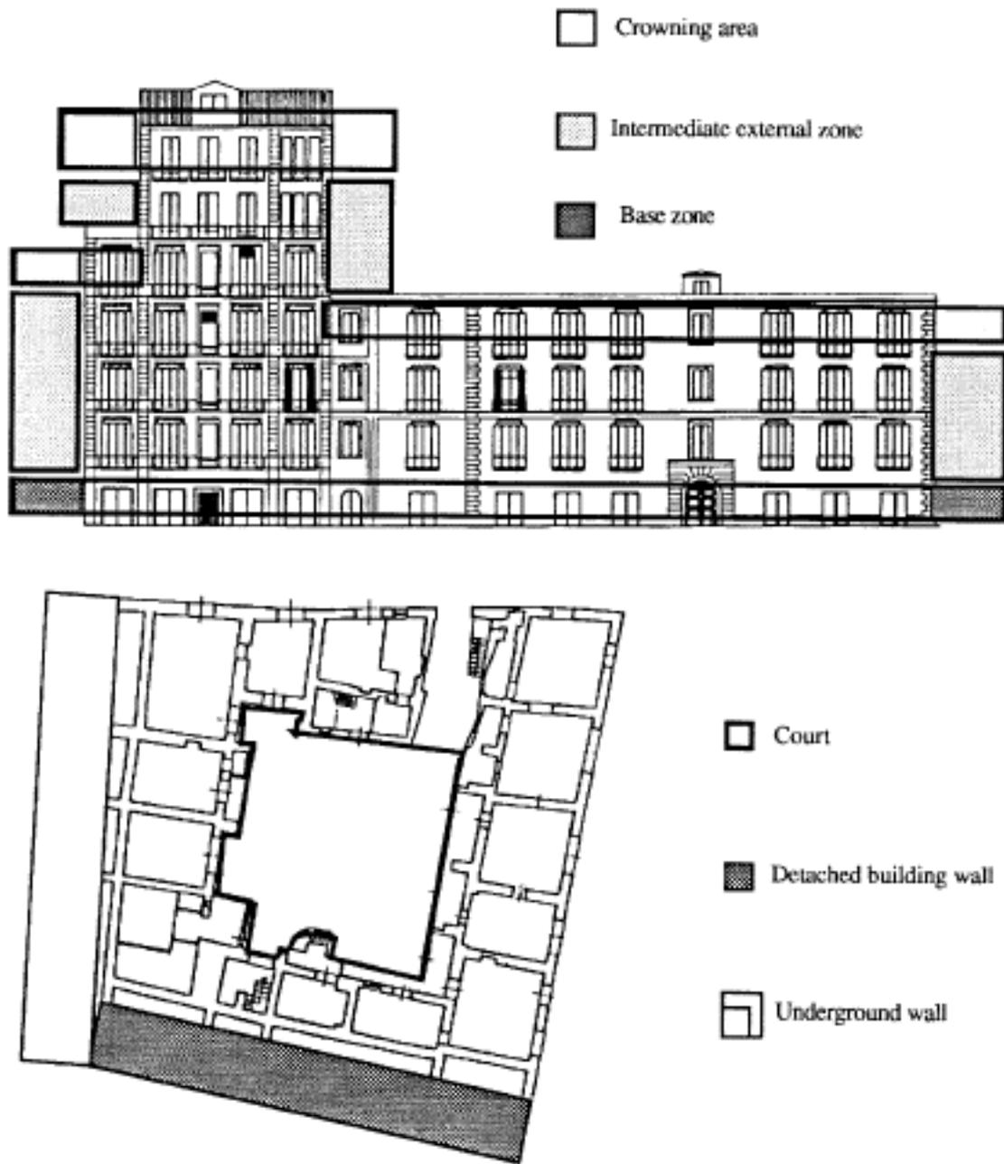
**FIG.7** Subdivision of the building according to the Expert System
