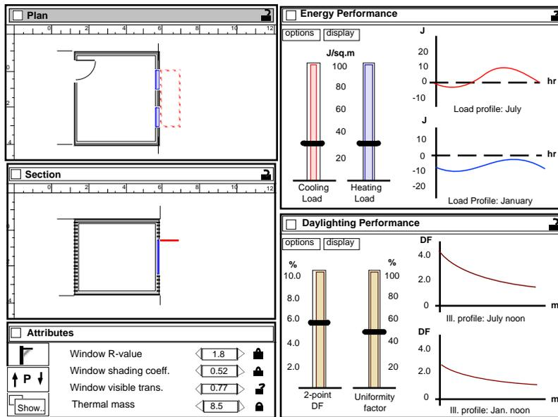
Figure 4d. Example of a formal transformation (change in room proportions) as the result of modification of the two-point daylight factor.
