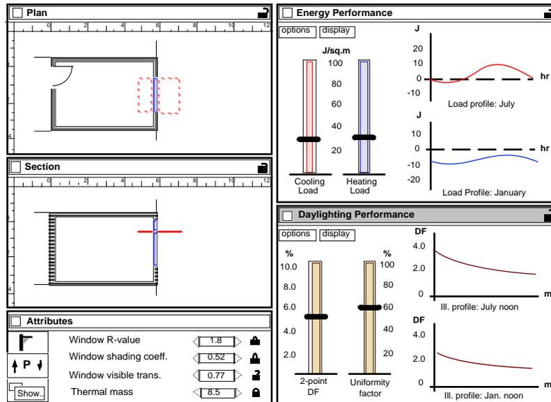
Figure 4c. Representation of component effects on daylighting performance. User can install/modify components and observe performance. Alternatively, changes in performance indicators are translated into design modifications.
