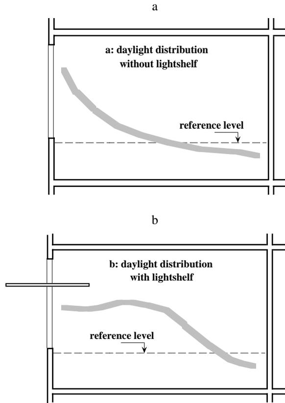
Figure 2. Schematic cross-section of a side-lit room without light reflector (a) and with light reflector (b) along with the corresponding curves of light distribution along the section line on a horizontal reference plane (after Mahdavi and Berberidou, 1992).
