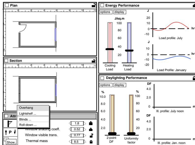
Figure 4b. Interface for simultaneous form generation and performance evaluation. Separate windows display geometrical attributes, component attributes, and various performance indicators (daylighting, energy).
