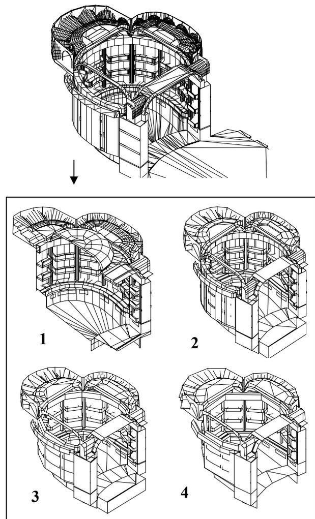
**FIGURE 1.** A completely modelled part of the GTB and the model simplifications (mod 1 - mod 2 – mod 3 – mod 4 ).
