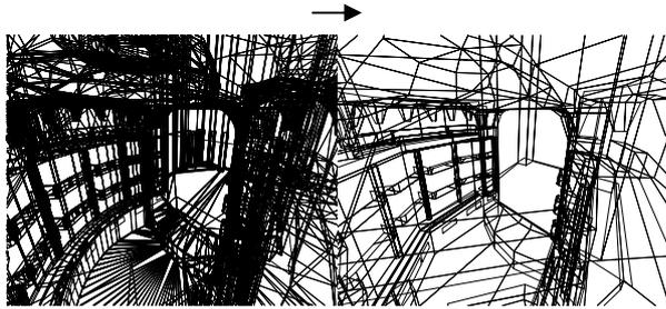
FIGURE 2. From the initial model (26696 facets) to the final simplified model (811 facets)
